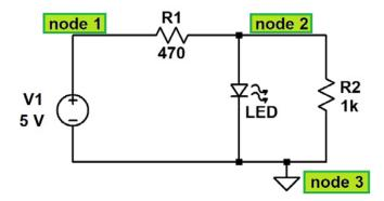
**3.1** The voltage drop across R1, R2, and LED can be measured using the M1K board by making wire connections between the circuit and M1K board pinouts.
