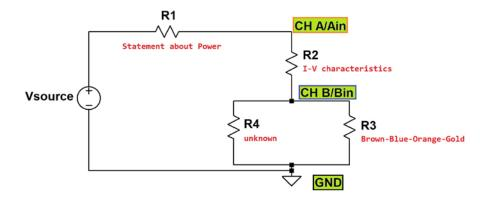
**2.1** The power absorbed by resistor R1 is 4.3 mW when 1.693 mA flows through it. Note: 'm' stands for milli. What is the value of R1?
