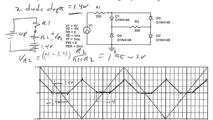
e. (3 Pts) For part b. What is the approximate voltage across D3 at the following times? Mark the schematic to indicate the polarity you used for these answers. (5pts)
