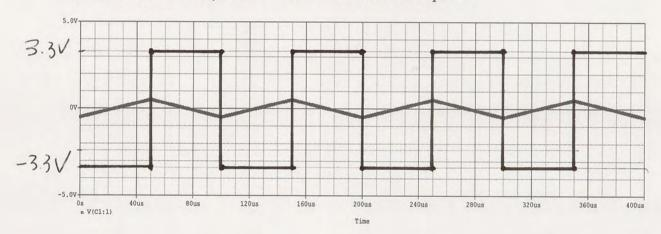
e. {4 pts} The input voltage is shown below. Solve for and sketch the output voltage for circuit C with  $R=100\Omega$  and  $C=0.047\mu F$ . Same scales as in part b.
