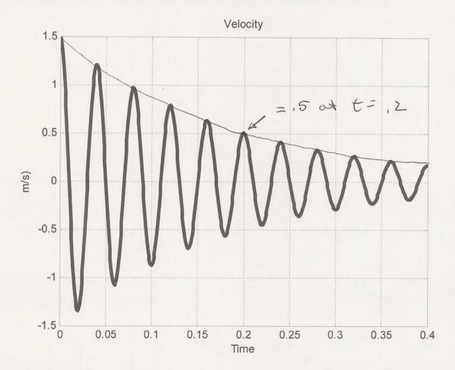
where the horizontal scale is time (0.05 sec per division) and the vertical scale is velocity (0.05m/s per division).
