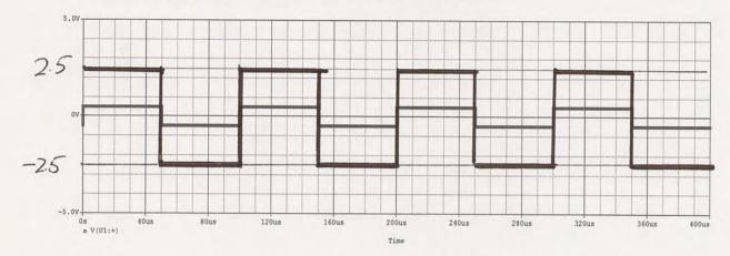
d. {4 pts} The input voltage is shown below. Solve for and sketch the output voltage for circuit D with C=.033 $\mu$ F and R=5k $\Omega$ . Same scales as in part b.
