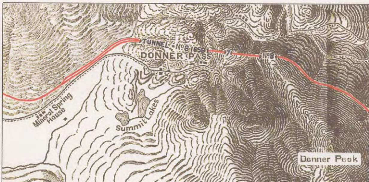
Topographic map of Tunnel 6's location (note also tunnels 7 and 8 to the east). This comes from the Manual for Railroad Engineers , 1883 and was drawn by Samuel Montague and Lewis M. Clement CPRR Chief and Ass't Chief engineers responsible for building Tunnel 6 and the CPRR line. "Summit Lakes" is now just Lake Mary which turned the two lakes into one with a railroad built dam to store water for steam powered locomotives.
