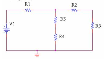
Given: V1=5 volts. R1=  $50\Omega$ , R2=  $1500\Omega$ , R3=  $2000\Omega$ , R4=  $680\Omega$ , R5= $430\Omega$
