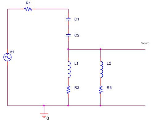
Consider the above circuit and apply your knowledge about the behavior of capacitors and inductors (i.e., open or short circuits at very high or very low frequencies).
