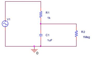
What type of analysis (simulation) would you have to run to determine if this altered circuit is a high or low pass filter? (Circle the best answer.)
