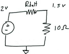
b.) (3 pts) Suppose that you measure the battery voltage while it is discharging into the 10 ohm resistor and find it to be 1.5V. What is the battery's resistance?
