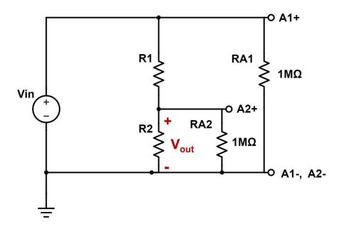
Under which conditions do we need to be concerned that the input impedance of channel 2 (RA2) will noticeably affect the voltage measurement across R2? [3 points: 1 for identifying voltage divider; 1 for identifying significance of parallel resistance; 1 for conditions for R2]
