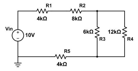
**Q1.1)** Find the voltage across R3. [4 points: 1 pt for  $R_3 \mid \mid R_4$ ; 2 pts for voltage divider equation; 1 pt for correct numerical answer]
