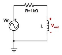
The formula for the corner frequency of a first-order filter with a resistor and an inductor is  $f_c = \frac{R}{2\pi L}$ . Solving for L with  $f_c$  = 6kHz and R = 1k $\Omega$ ,  $L = \frac{R}{2\pi f_c} = \frac{1k\Omega}{2\pi*6kHz} = 26.5 \, mH$
