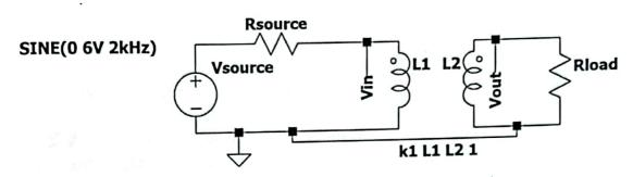
Assume L1 and L2 form an ideal transformer with full coupling. The transformer has these specifications: a=3, L1=5mH
