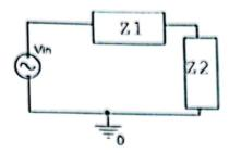
This circuit shown above has 2 complex impedances, Z1 and Z2, connected as shown.
