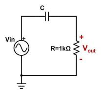
Using the value determined for the corner frequency in Q2.1, calculate the capacitance C required for the filter. [3 points: 2 for correct formula; 1 for correct numerical answer for C (if Q2.1 was correct)]
