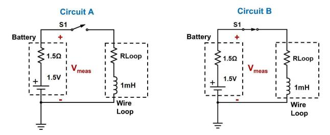
If the voltage across the battery is measured while the motor is operating, the plot below is observed on the oscilloscope: when the circuit is open (A), 1.5V is measured and when the circuit is closed (B), 0.75V is measured.
