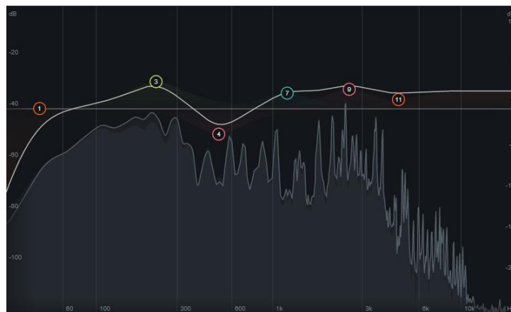
Figure 14 – Equalizer tool in the DAW Reaper using six filters (denoted by circles) to modify the audio signal from a guitar
