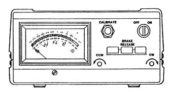
Figure 1 Control Unit - Front Panel
