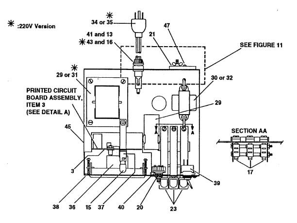
Figure 9 T-2X Control Unit Inside-Top View
