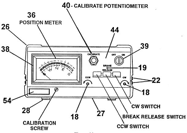
Figure 11 Front View of T2X Control Unit
