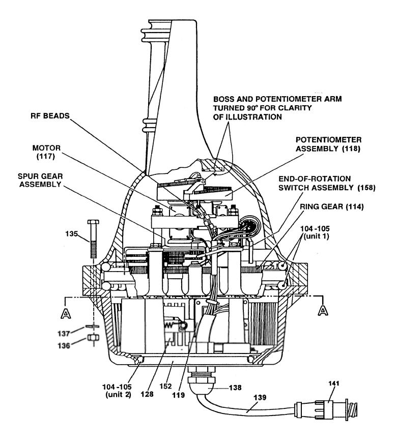
Figure 12 Inside View of T-2X Rotator
