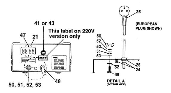
Figure 10 Rear View of T2X Control Unit
