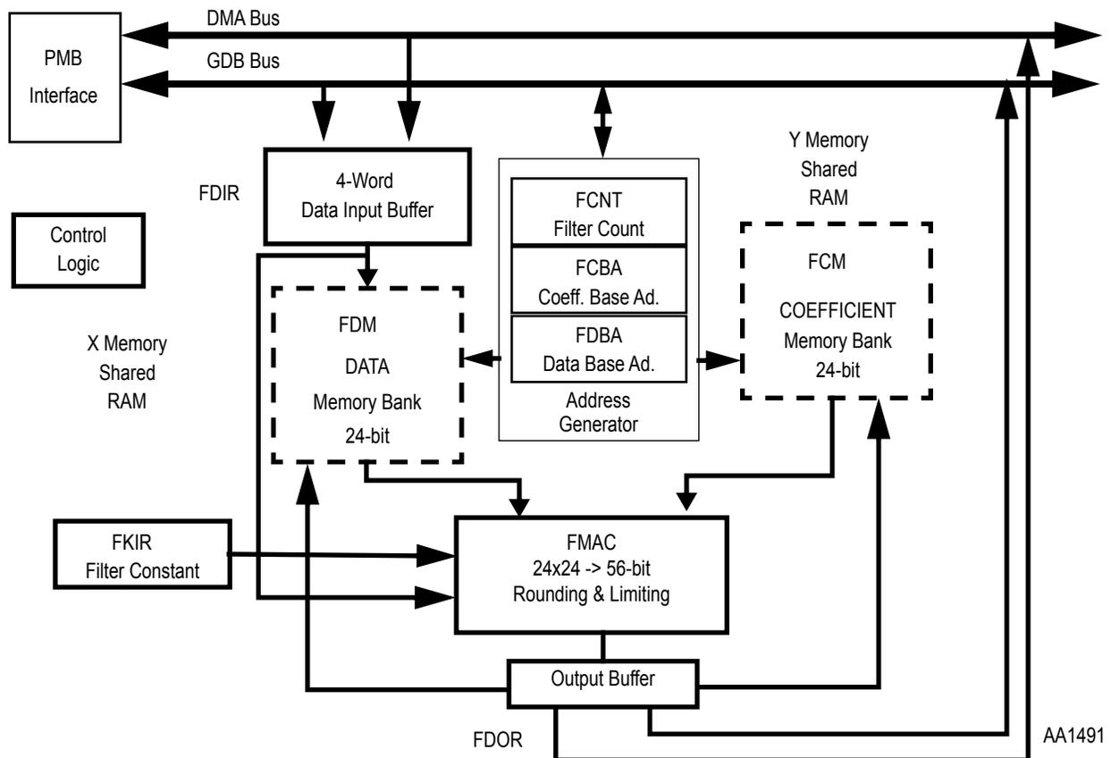
Figure 1-1. EFCOP Block Diagram
