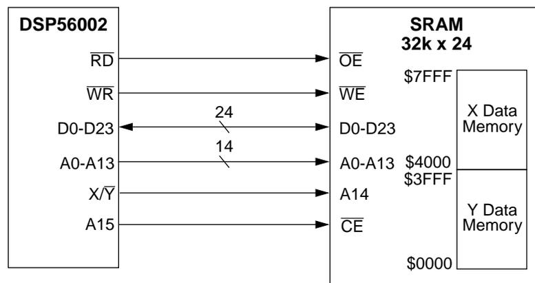
Figure 2-1 DSP56002 Interface to External SRAM
