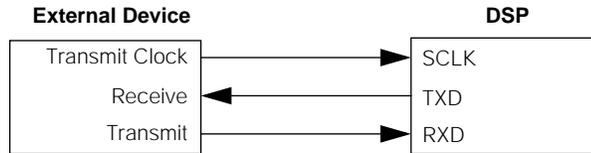
**Figure 1.** SCI Connections
