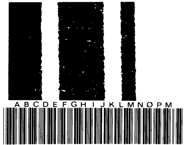
Figure 15. Photomicrograph of Photolithographic Label
