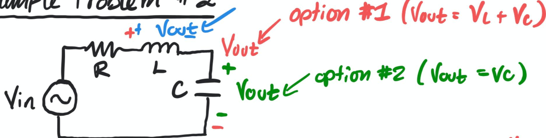
option #1 ( $V_{out} = V_L + V_C$ )option #2 ( $V_{out} = V_C$ )
