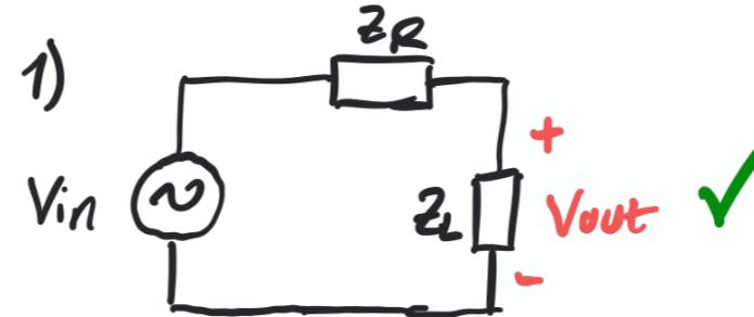
$$2) V_{out} = V_{in} \frac{Z_L}{Z_L + Z_R} \quad \checkmark$$
