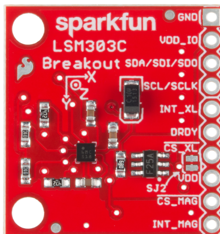
Figure 5.15 - The 3-axis Acceleration Module (or compatible version). GND and VDD_IO are the ground and +3.3V connections, SDA and SCL are self-explanatory. No other pins are used.
