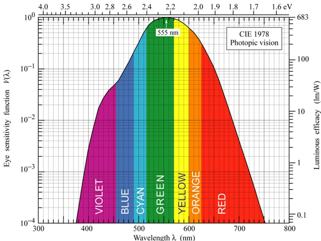
Fig. 16.7. Eye sensitivity function,  $V(\lambda)$ , (left-hand ordinate) and luminous efficacy, measured in lumens per watt of optical power (right-hand ordinate).  $V(\lambda)$  is maximum at 555 nm (after 1978 CIE data).
